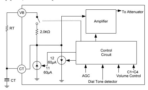
CT Attenuator Control Block Circuit
